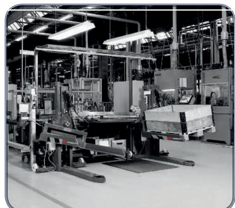
The tilt function reduces the reach distance for the operator. The forks can be tilted up to 40 degrees (both left and right).
